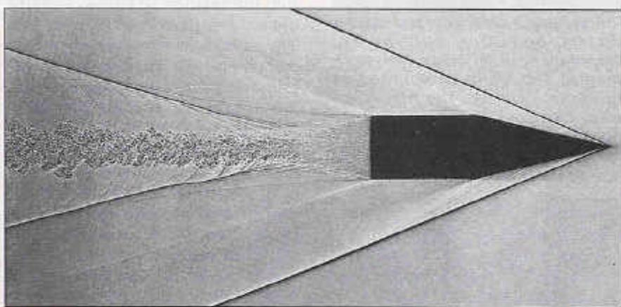
*Acoustic sensors can detect the origin of a passing projectile by discerning the leading-edge shock wave pattern as it fans out from the nose of the object. This shock wave is compared to the weaker recompression shock wave that trails the projectile.*
